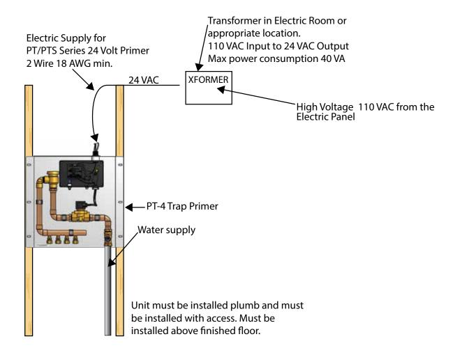
24V SURFACE MOUNT Cabinet Size: 12" x 12" x 4" MODELS: PTS-4 Thru PTS-12 MODEL: PTS-1320 MODEL: PTS-2130 24V FLUSH MOUNT
